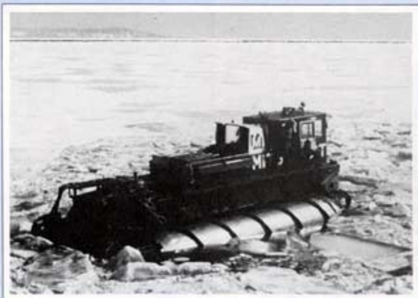
AST amphibian: The 11-metre-long (36-ft.) AST gets its name from the two cylindrical screw rotors which support the 11-tonne craft.
